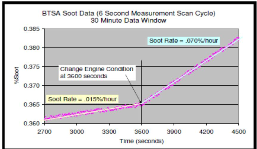
*A soot measurement is acquired every 6 seconds. Soot accumulation rate can be determined based upon the trend provided by this 6 second data.*
