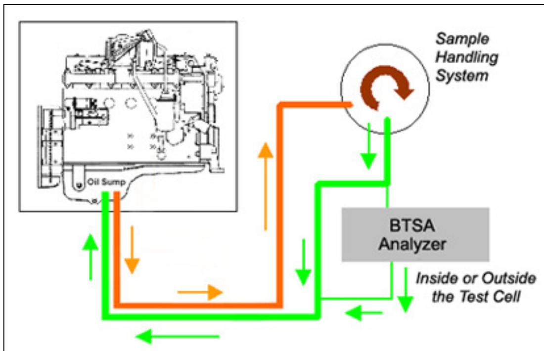
The BTSA measures the engine's soot concentration during dynamometer testing. As the oil flows through the hydraulic circuit, it is optically scanned to accurately determine the instantaneous soot concentration. The sample is returned to the engine sump, unaffected by the measurement.
