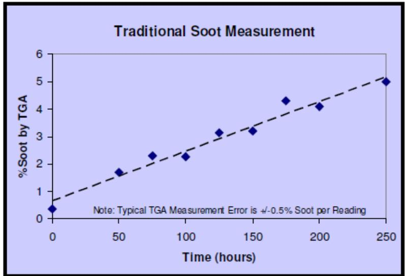
*Soot Measurements Using Laboratory TGA Methods*
