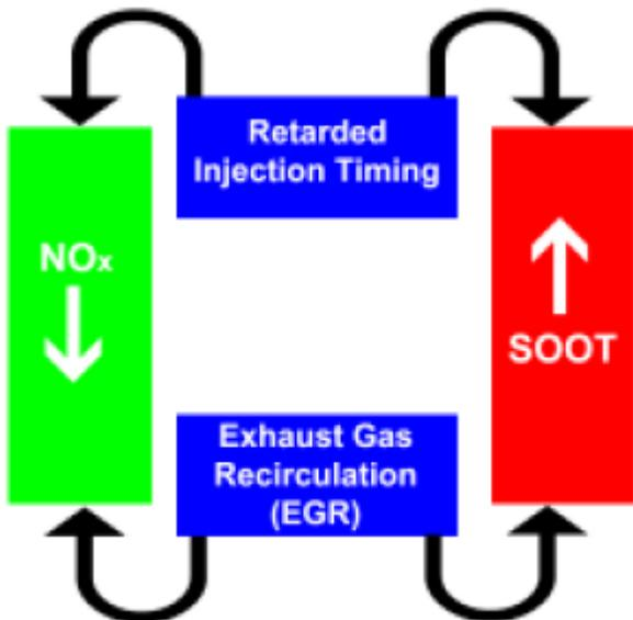
Worldwide regulation of lower exhaust emissions has resulted in retarded fuel injection and the implementation of EGR to control NOx. Both of these NOx control strategies can cause the engine to produce more lubricant oil soot. This has posed a serious challenge to engine developers and oil companies.
